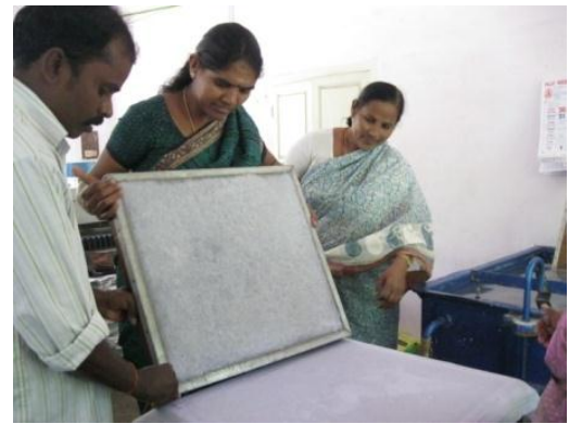
Uni-Vat Machine- for making recycled paper sheets
